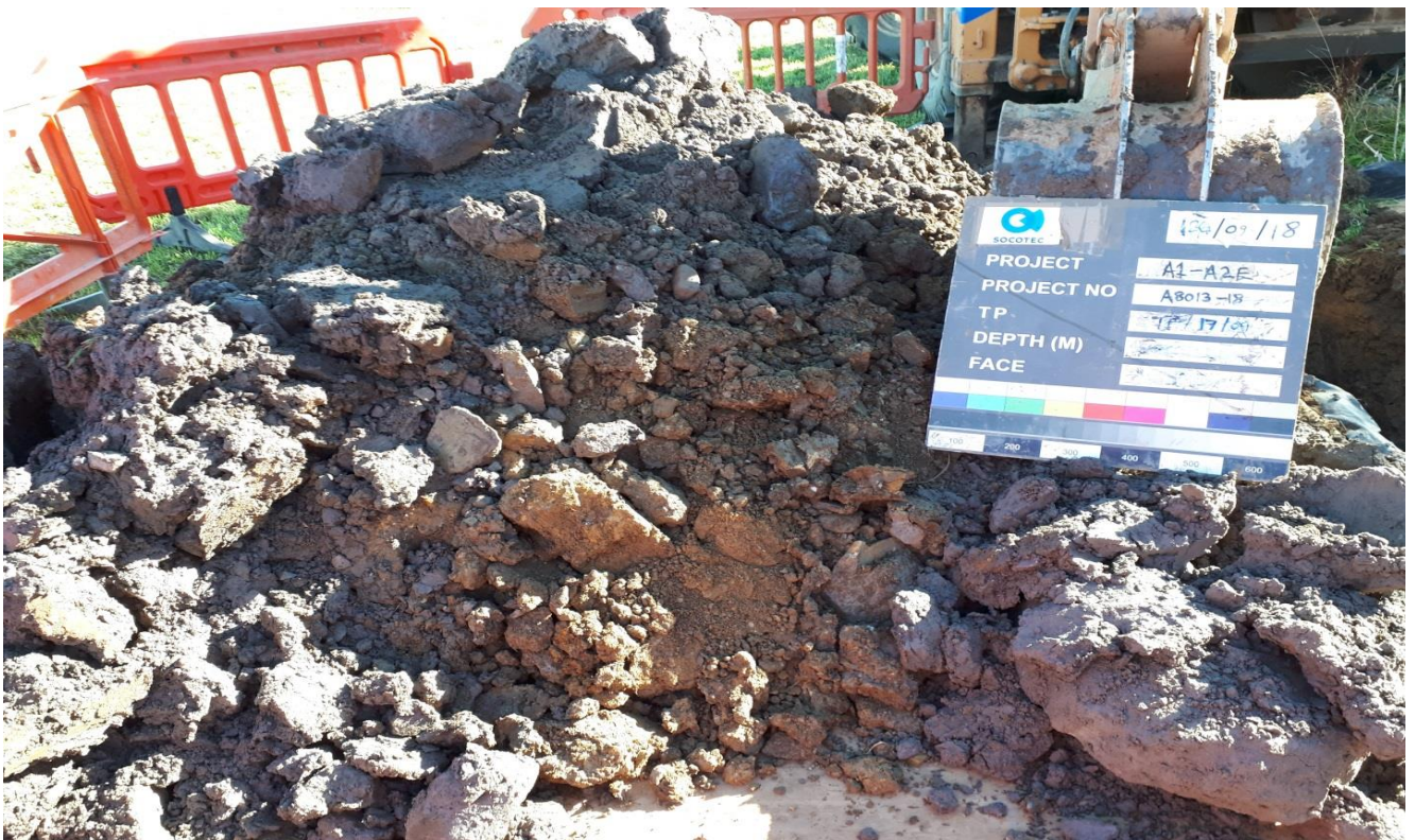
TP/17/09A Spoil 2.30m
