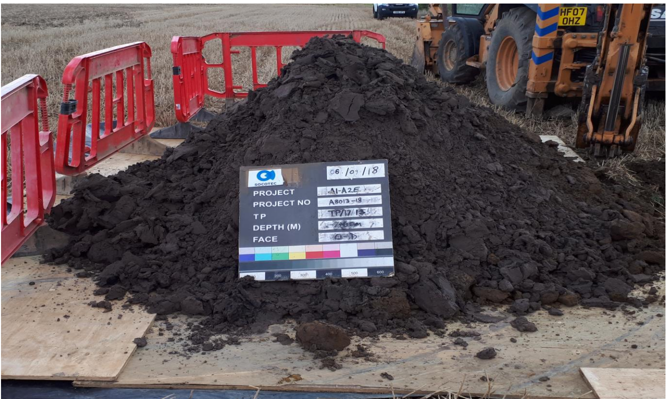
TP/17/15 Spoil 2.60m
